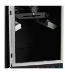
Optional UV lamps for overhead illumination. 254/365nm UV; 95-0021-12 (115V) and 95-0021-10 (230V)
